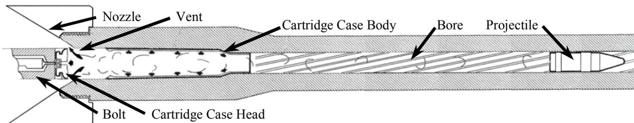
Figure 1: Schematic of a blowback bolt-operated RAVEN shortly after commencement of the venting.
