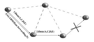
Figure 4. Data flow and alarm: A sends data and receives an ALARM from C that D does not forward.
