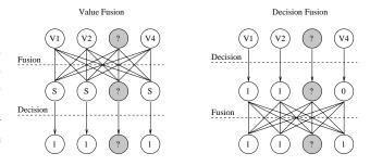
Figure 2: Two approaches for fusion. The grey sensors are faulty and have indeterminate behavior.
