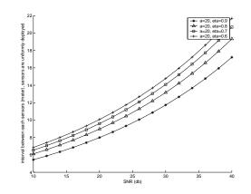
Fig. 4. relation between maximum sensor interval and SNR, the confidence level
