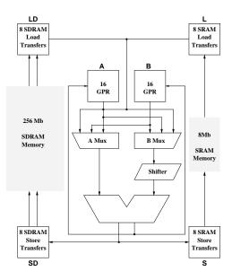
Figure 1: Micro-engine architecture
