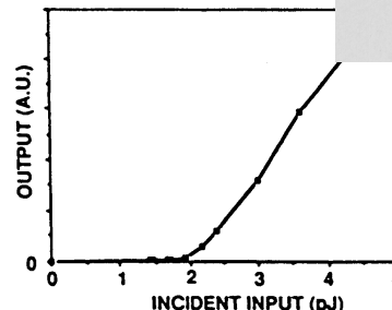
Fig. 5. Output at 865 nm vs. incident input energy for a 0.4 \times 0.4 \mu\text{m} microlaser.
