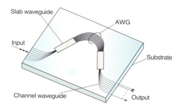
Waveguide pattern of AWG multi/demultiplexer chip
