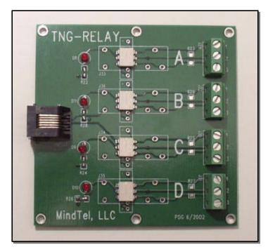
Screw terminal connections are optional, as is the 6-6 modular jack.
